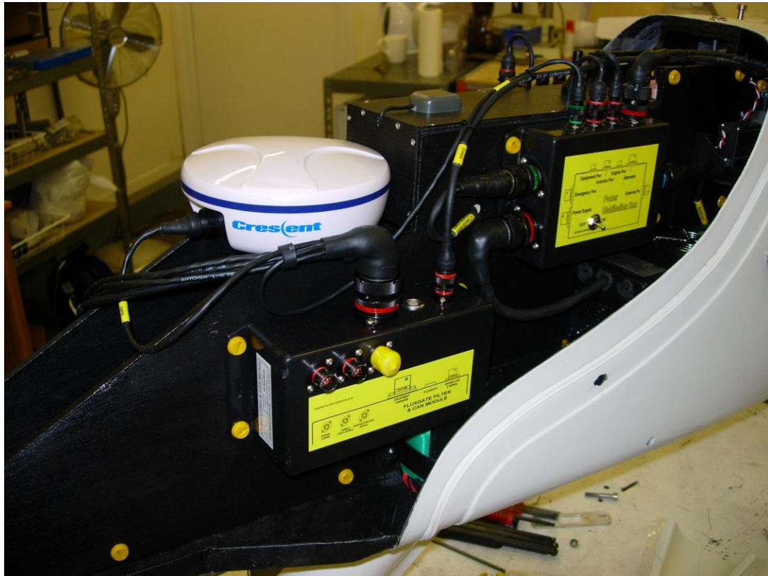
Prion Mk 3 On-board electronics, nose cowling removed.
