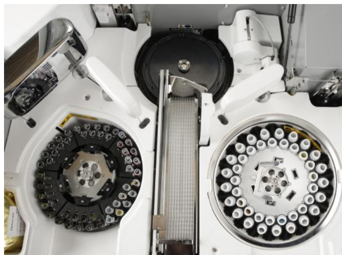
Indiko Plus system has a sample disk for up to 108 samples : 9- or 18-position sample racks, max 6 racks. Reagent disk in Indiko Plus has positions for 42 reagents.
